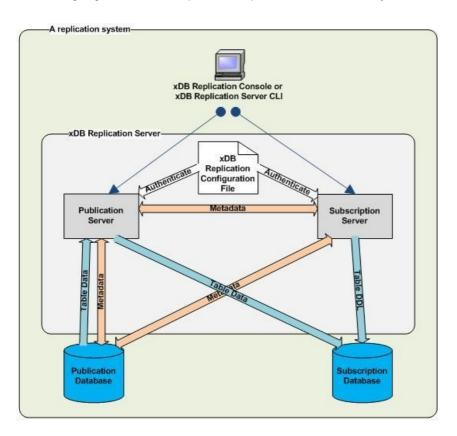
The following diagram shows the components of Replication Server and how they're used to form a complete, basic, multi-master replication system.
