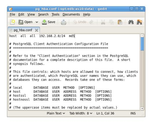
You might also need to manually modify the pg\_hba.conf file to allow connections between the PEM server and other components. For example, if your PEM-HTTPD installation isn't on the same host as the PEM server, you must modify the pg\_hba.conf file on the PEM server host to allow PEM-HTTPD to connect to the server.
