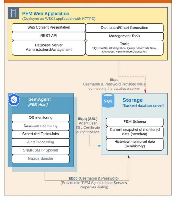
The PEM server consists of an instance of Postgres, an instance of the Apache web server providing web services to the client, and a PEM Agent. PEM uses a server-side cryptographic plugin to generate authentication certificates.
