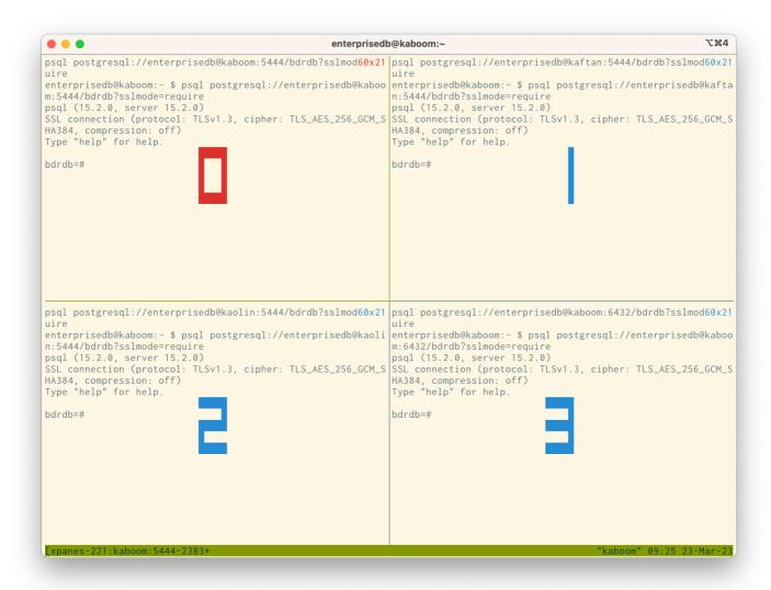
To switch the focus between the panes, you can use **Control-b** and the cursor keys to navigate between them. Or you can use **Control-b** followed by **q** and the number of the pane you want to focus on. We'll show both ways.
