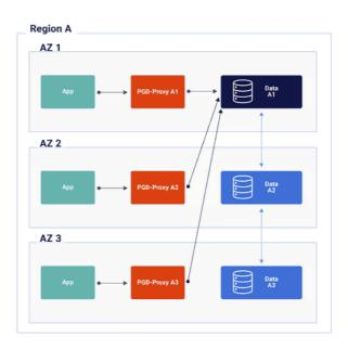
The EDB Postgres Distributed for Kubernetes operator can control the scheduling of pods (that is, which pods go to which data center) using affinity, tolerations, and node selectors, as is the case with EDB Postgres for Kubernetes. Individual scheduling controls are available for proxies as well as nodes.
