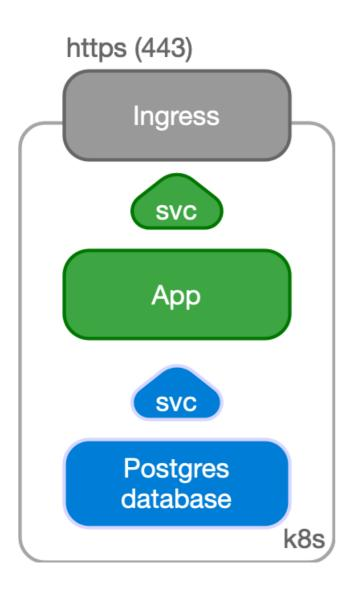
The application, normally stateless, is managed as a standard deployment, with multiple replicas spread over different Kubernetes nodes and internally exposed through a ClusterIP service.
