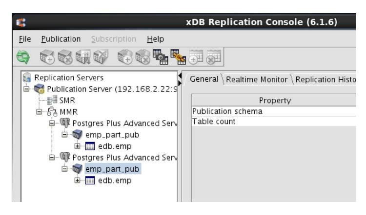
You can now keep the partitioned table synchronized on the primary nodes of the multi-master replication system.
