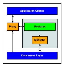
The consensus layer is an external entity where Harp Manager maintains information it learns about its assigned Postgres node, and HARP Proxy translates this information to a valid Postgres node target. Because Proxy obtains the node target from the consensus layer, several such instances can exist independently.
